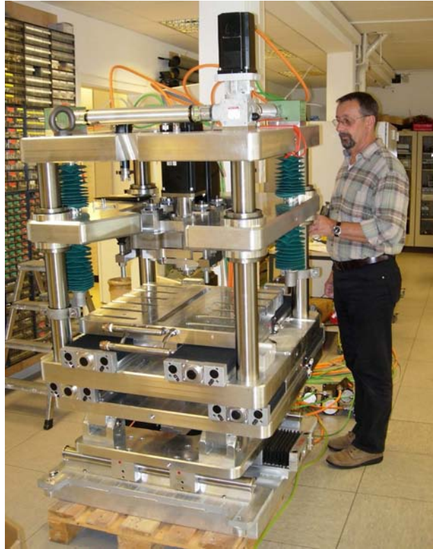
Figure 6: The in-situ friction stir welding apparatus FlexiStir.
