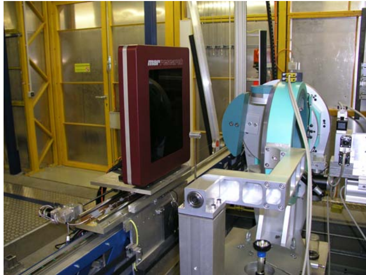
Figure 4: The Mar555 detector mounted on carrier 1 of the detector portal.
