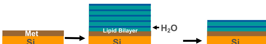
Figure 1: Supposed layer composition after the different treatments.
