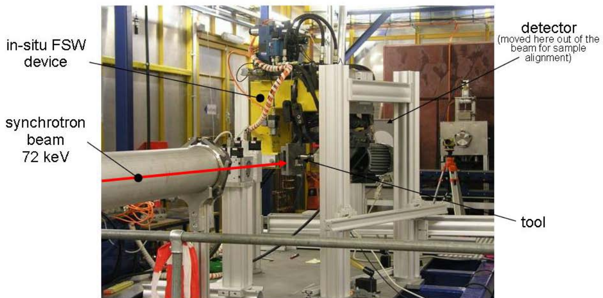
Figure 1: View of the experimental setup with in-situ FSW device for high-energy SAXS studies at HARWI II.
