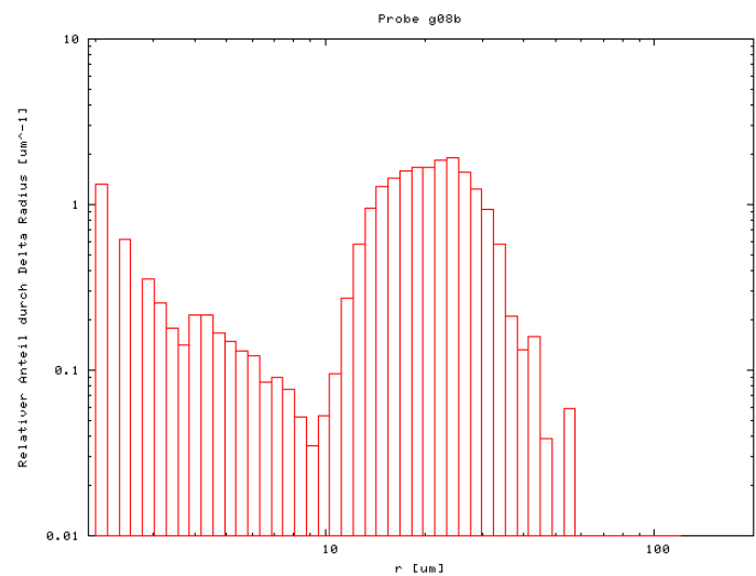
Figures: Top: Two representative samples with different pore size distributions. Bottom: left: Tomographic rendering for a bi-continuous network of artificial bone + bimodal pores; right, typical pore size distribution for a sample with a bimodal size distribution. The bar stands for approximately 40 microns.
