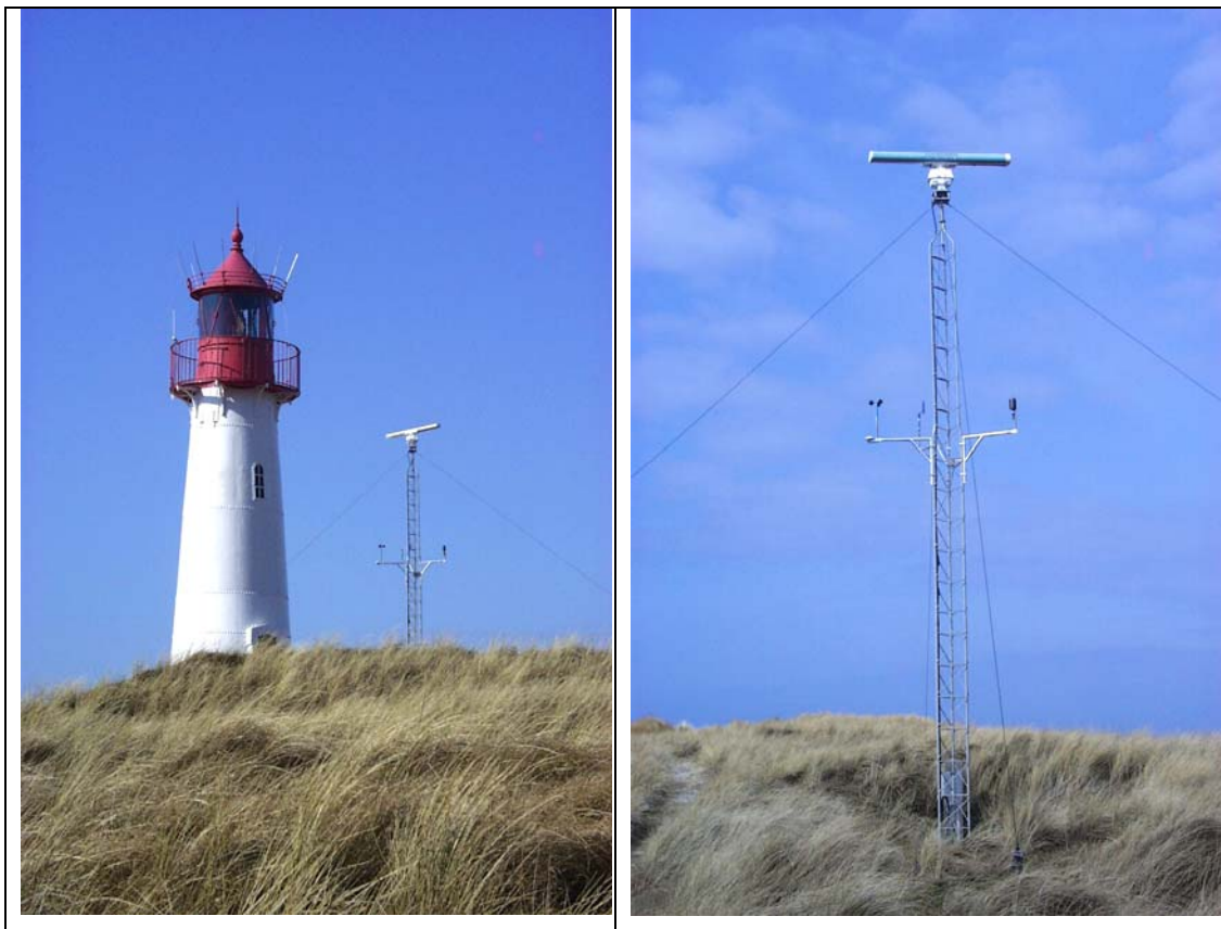
Figure 4-3. The left image presents the radar of List West station, next to the lighthouse of the List West, and on the right the mast of the radar Furuno FR 1201, on the top and the meteorological station few meters lower (Image source: KOR, GKSS).
